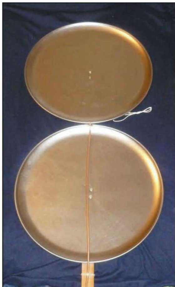
Photo A. A planar disk antenna ... built from two dollar-store pizza pans!
